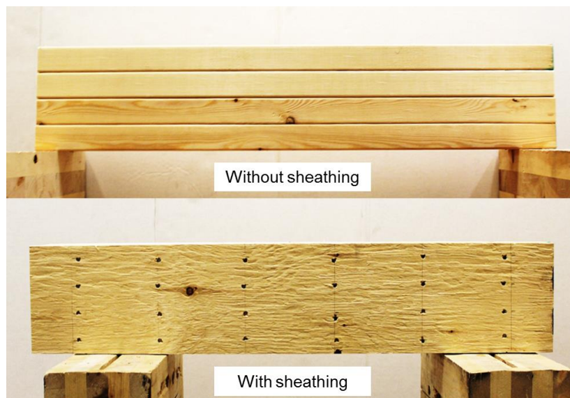
Figure 3 Specimens for NLT bending-shear test
