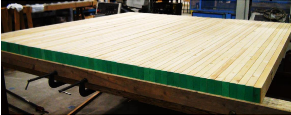
Figure 5 NLT wall specimen during manufacturing
