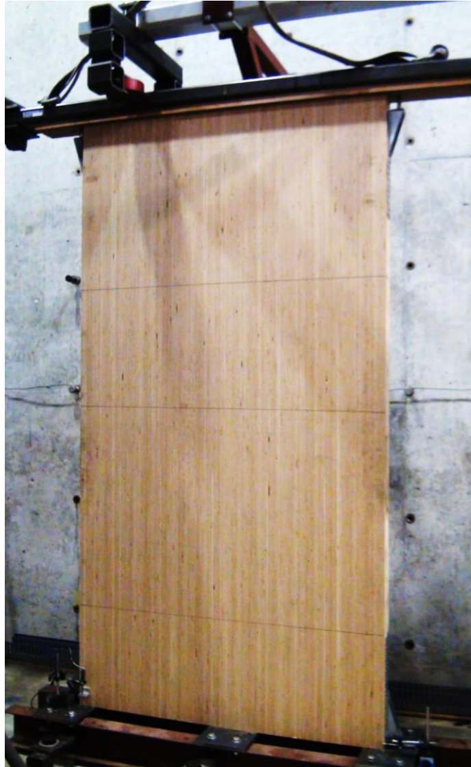
Figure 10 Post laminated LVL shear wall test setup
