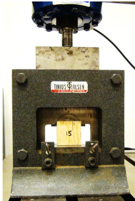
Figure 8 Block shear test setup
