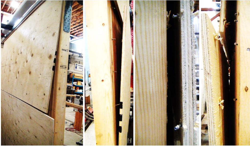
Figure 20 Failure of NLT walls with sheathing
