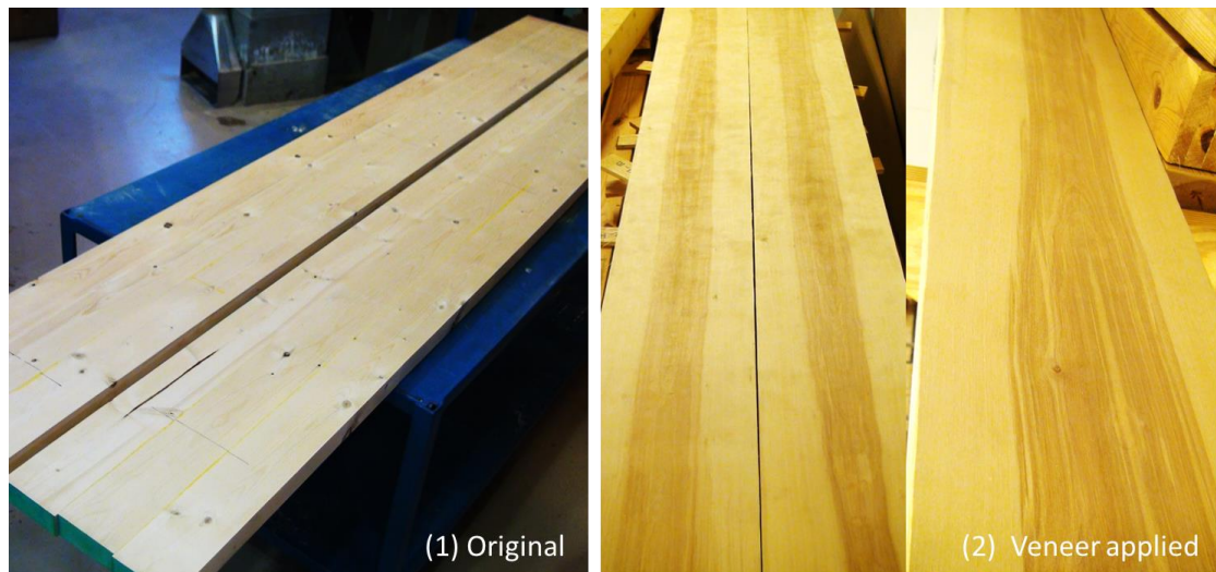
Figure 2 Appearance of the panel before and after veneer applied
