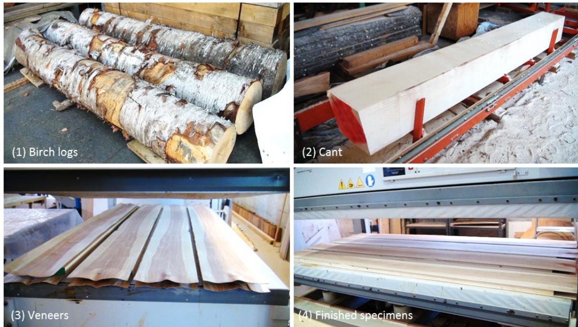
Figure 1 The process of specimen preparation
