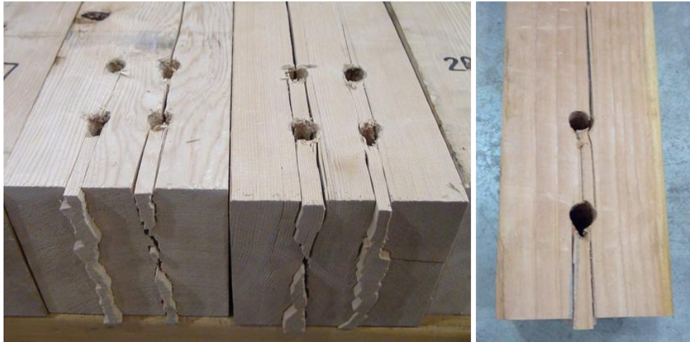
Figure 6 Row shear failures
