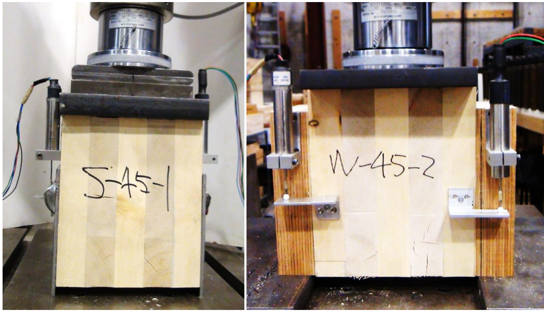
Figure 5 Setup for the intra-module connection test
